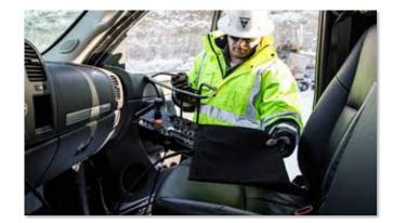
**THE SYSTEM** allows the operator to be located within a vehicle, such as a pickup, and seated on a mat-style seat switch to operate the attachment functions in work mode.
